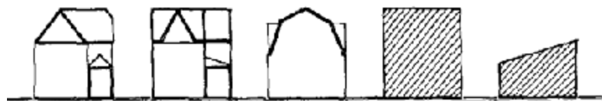
Roof shapes inconsistent with adjacent structures.
