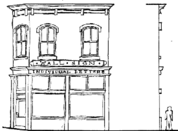
Wall signs appropriate for the historic overlay.
