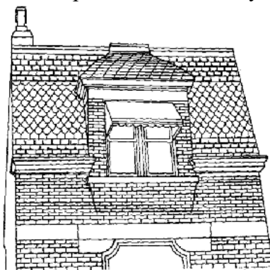
Example of an original mansard slate roof.
